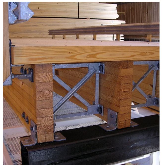
Close Up View of Model Bridge Steel Diaphragms
